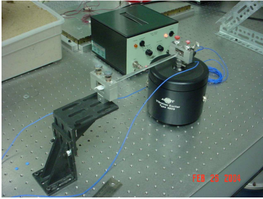
Fig. 5 Picture of the experiment setup for transverse vibration of pre-stressed silicon specimen
